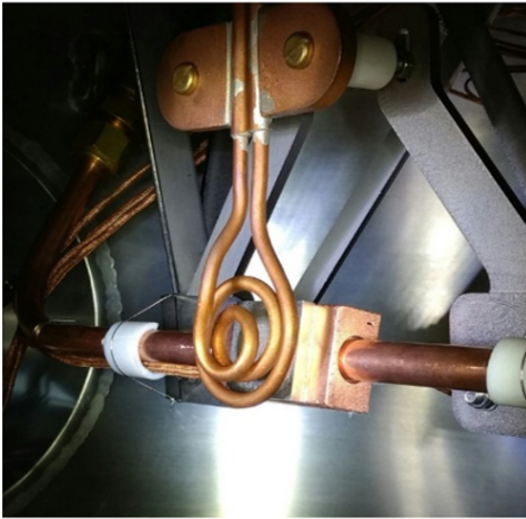
Fig. 4.5: (left) Photograph of sample mounted under induction coil within HIVE; (right) photograph of sample heated during a physical test.
